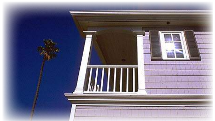
Second floor balcony at corner helps break down mass of flat wall.
